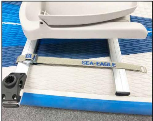
In summary, the strap loops around the rear bar rests on top of the front bar.
