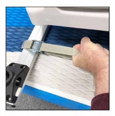
Tuck strap end into the back of the buckle for a clean finish.
