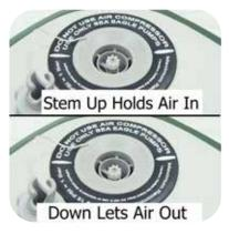
Press and turn the stem counterclockwise so it can pop UP. When the stem is up, the valve is closed and will hold air. To let air escape for deflation, press and turn the stem clockwise until locked open.
