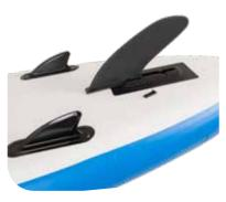
Slide the skeg into the base and secure with the clip. If a skeg will not slide into its base, do not force it. Refer to instructions on page 14.
