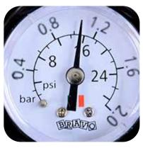
The pressure gauge will not begin to register until the board begins to get pressurized. Pump until the working pressure of between 12 and 14.5 PSI is reached. Do not exceed 15 PSI when inflating.
